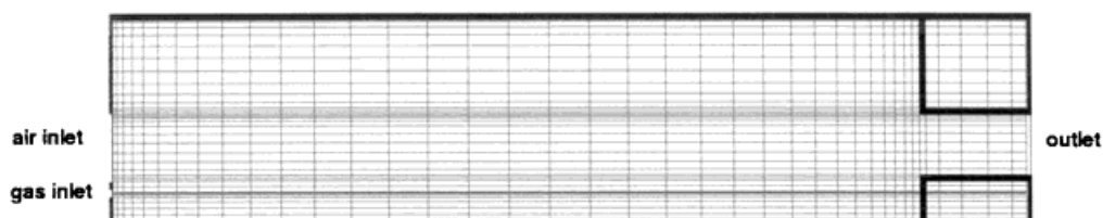
Figure 2. The symmetry plane of the furnace. Grid 42 \times 37 \times 27 .
